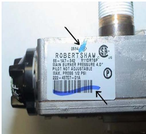
Valves that have been serviced in the field can be identified by a label that reads "05-NS35".
