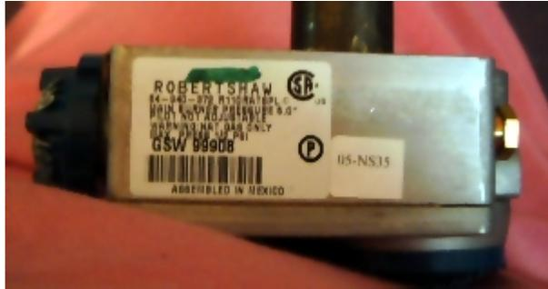
Unaffected valves on Bradford White, water heaters can be identified by a blue mark at the date code and through the UPC symbol. (See picture below.)
