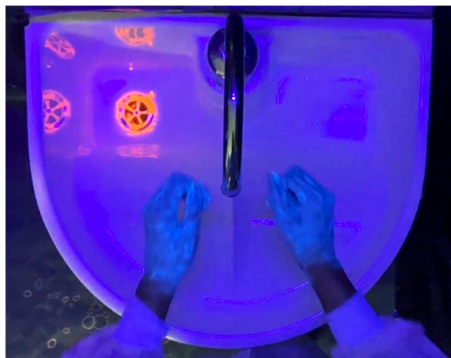
Figure 3: Orange Glo Germ™ oil on drain strainer and blue-white Glo Germ™ gel on participant hands at the barrier-free sink.
