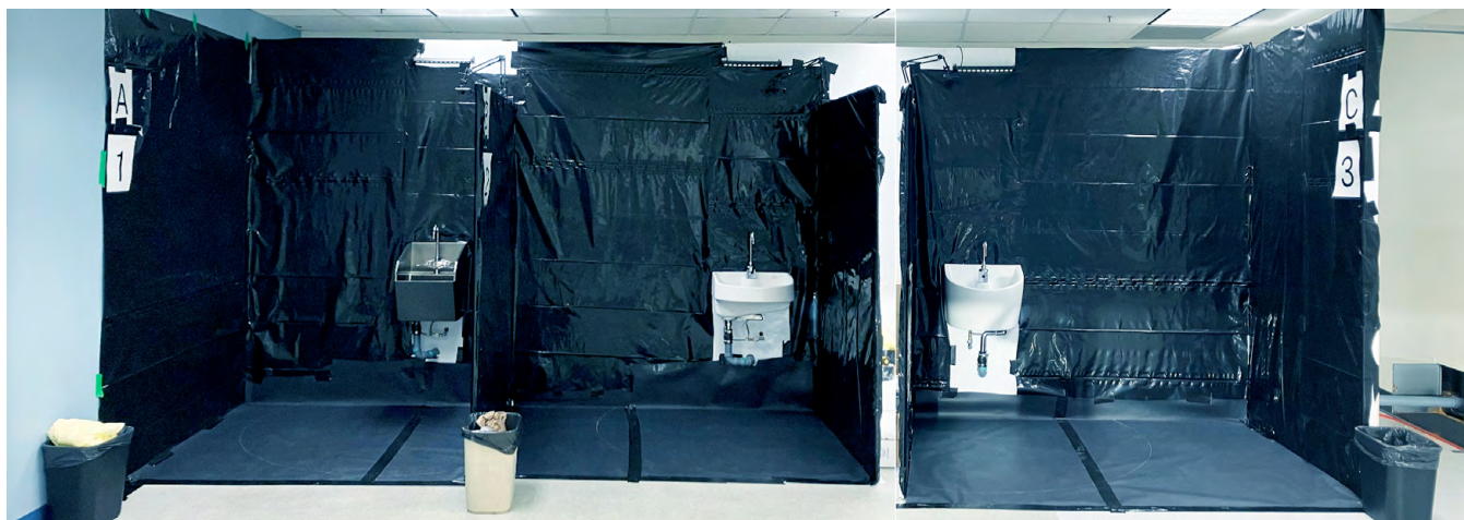
Figure 2: Photos of week 1 splash study cubicle setup with trough sink, barrier-free sink, and deep rounded sink from left to right.
