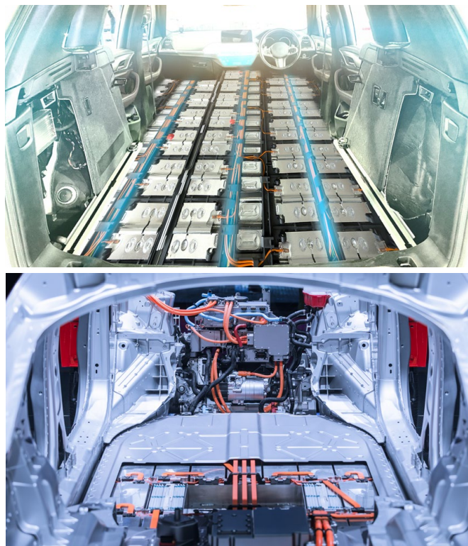
Figure 5: LIB packs with battery management system in EVs.
