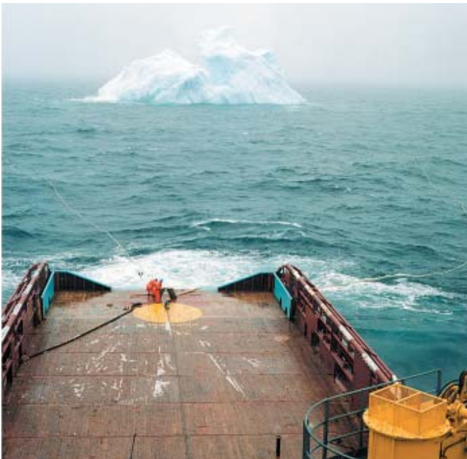
Outside St. John's, NFLD, encroaching icebergs are "lassoed" with a heavy cable and towed by a platform support vessel into a different trajectory.
